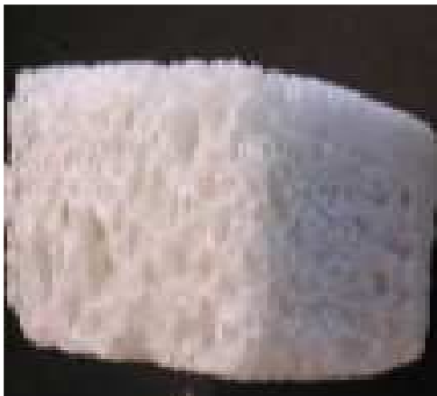
Figure 2: foam glass obtained by wet process
